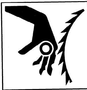
A.8.13 Fingers or hand entanglement — Cotton stripper cleaner drive
