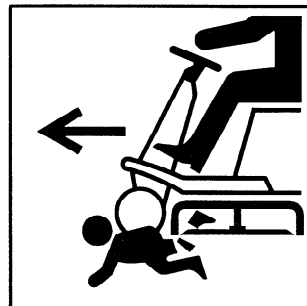
A.7.9 Dismemberment — Rear engine mower in forward motion
