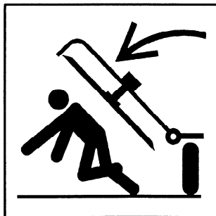
A.6.15 Crushing — Rotary cutter
