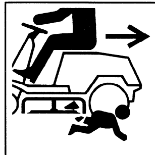
A.7.10 Dismemberment — Rear engine mower in rearward motion
