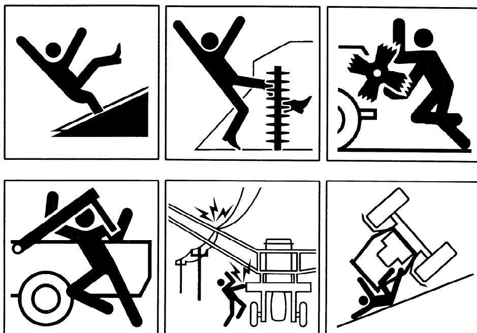
Figure D.16 — Examples of pictorials showing machines and hazard-creating major components
