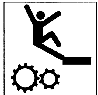
A.4.4 Falling into machinery — Rotating gears
