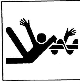
A.8.12 Arm or upper torso entanglement — Rotating auger
